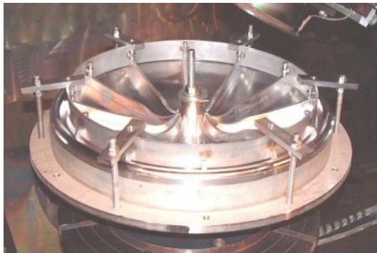
ANL 3-Spoke resonator end-plate with ribs calibrated for minimum df/dP
