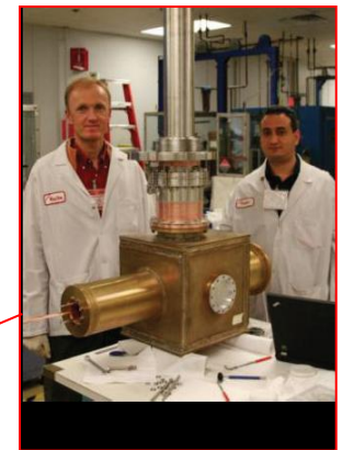
100 kW power coupler for 125 mA beam (IFMIF/EVEDA)
