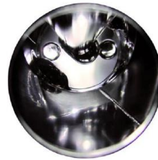
AFTER 12HRS OF EP 150µm Nb REMOVED
