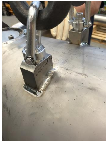
Residue on cavity surface
