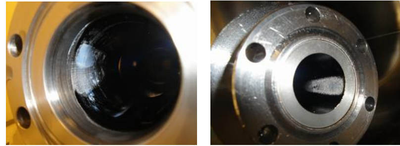
Vapor and gas build up in ports
