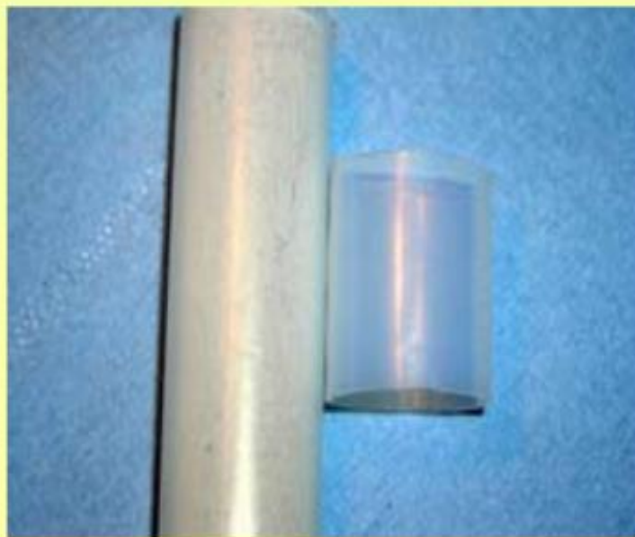
Tube before and after ethanol rinsing
