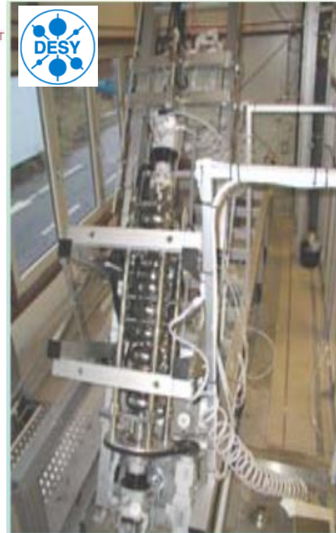
Cavity assembled to EP stand
