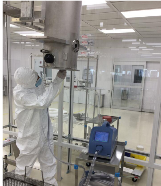
ISO 5 /Class -100 Surface particle counts of QWR
