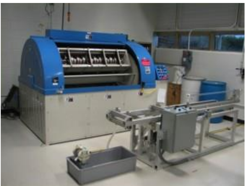
The tumbling machine can hold two nine-cell accelerating cavities, rotating them up to 115 turns per minute. The rinsing device (right) washes the media out. Cavities must be absolutely free of any extraneous material after tumbling.
