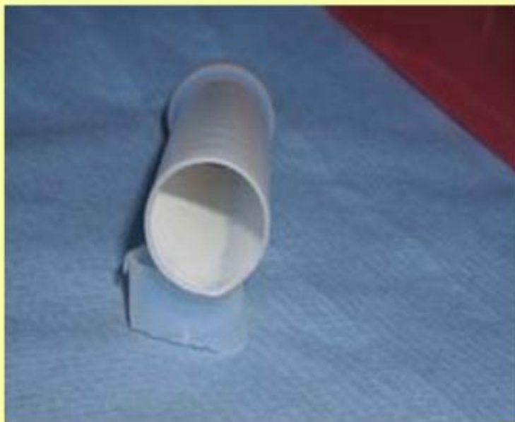
Tube with a thin sulphur layer
