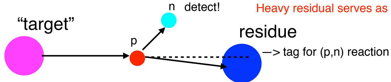
Efficient measurements can be performed even with RI beam
