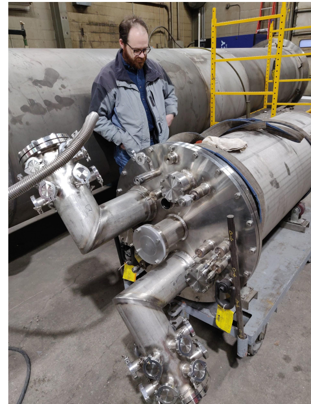
At Ability Engineering, Chicago: vacuum jacket has passed its leak check.
