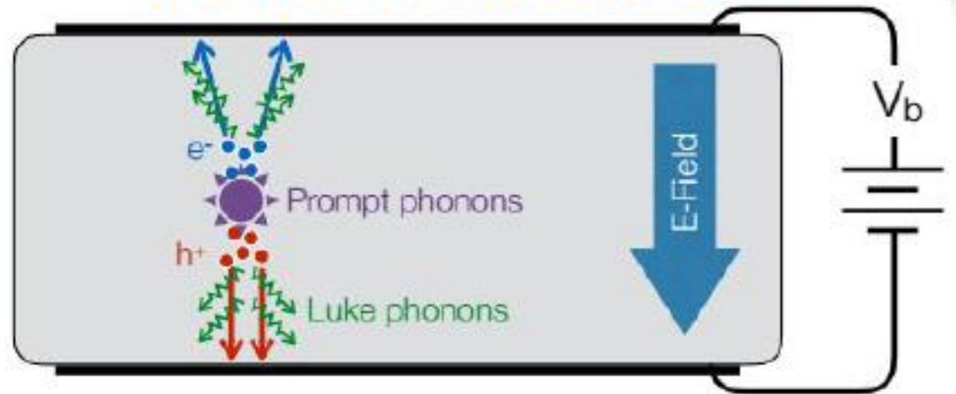
$$E_t = \underbrace{E_r}_{\text{Primary recoil energy}} + \underbrace{n_{eh}qV_b}_{\text{NTL phonon energy}}$$
