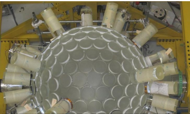
Light guides bonded & annealed in radon reduced air oven
