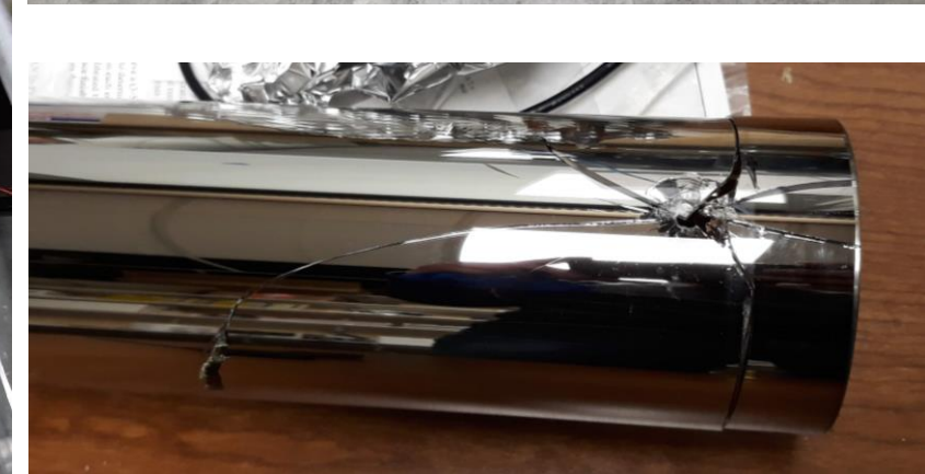
Glass guide broke during disassembly
