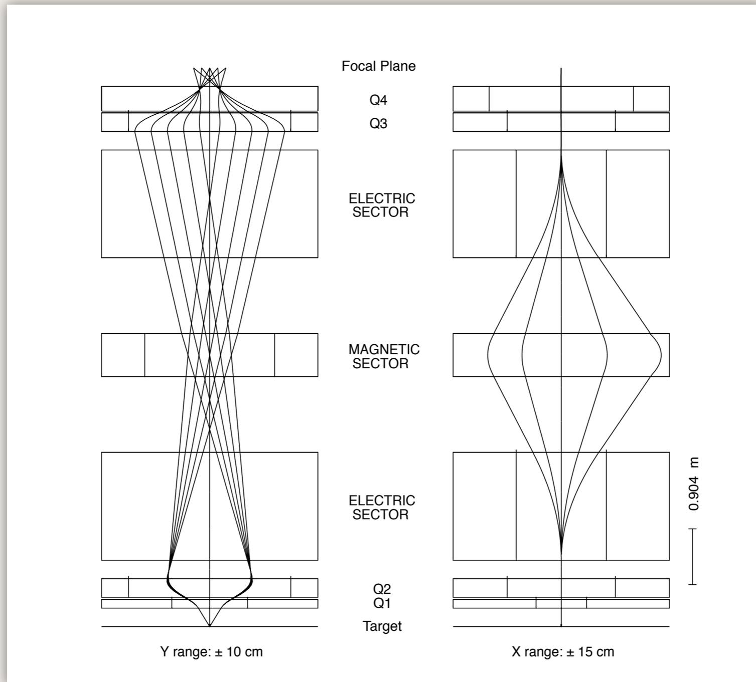
Single Mass, Vertical Angles of  $0, \pm 2^\circ$ , Energies Deviating from Central Value by  $0, \pm 7.5\%$  and  $\pm 15\%$
