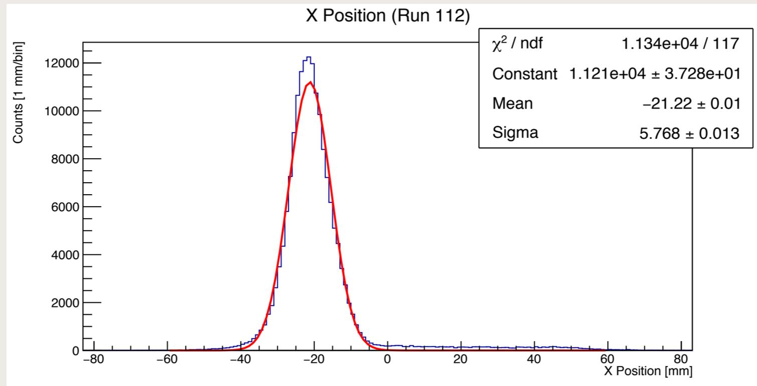
Set for  $^{197}\text{Au}^{9+}$ , observed single mass peak, no background in hour-long run with  $10^9$  ions/s on target implying hardware beam suppression  $> 10^{12}$
