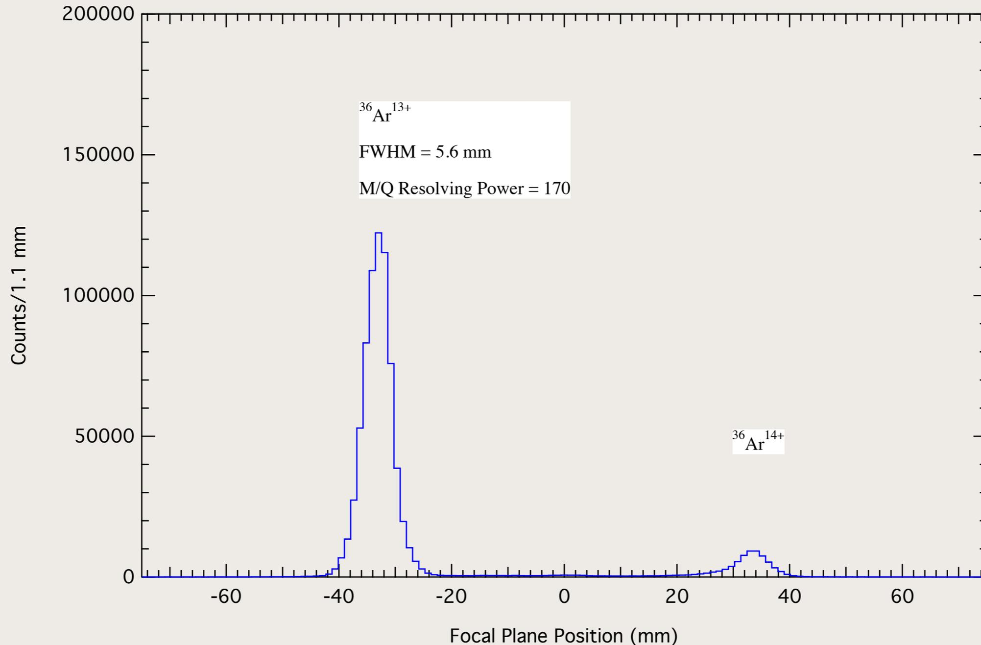
Measured mass/charge dispersion & resolving power consistent with ion optical calculations
