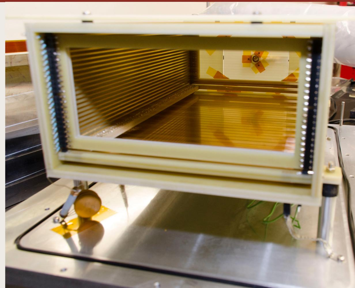
Ionisation chamber tested with alpha and fission sources on bench
