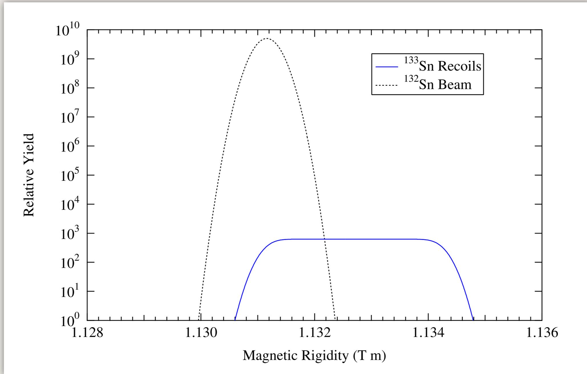
$d(^{132}\text{Sn}, p)^{133}\text{Sn}$  at 6 A MeV with  $100 \mu\text{g cm}^{-2}$   $(\text{CD}_2)_n$  target; smallest achievable beam energy spread; protons from 90-170 deg in lab
