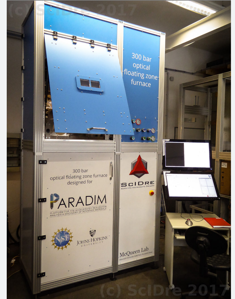
High pressure floating zone – Gas Pressures up to 300 bar
