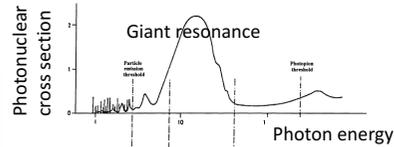
Fig. 1. Total photonuclear cross section as a function of the photon energy  $k$  [17].
