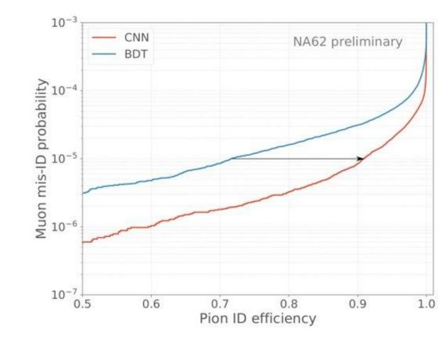
Pion acceptance can be increased from **72** % **to 92** % over the 15 to 50 GeV/c (muon mis-id 10<sup>-5</sup>)
