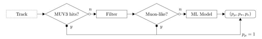
Data driven approach, training, validation and testing samples selected directly from the data. Independent test sample (*minimum bias*) used for the final evaluation.
