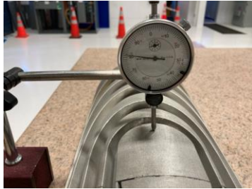
Control of SMCT coil end parts by micrometer on granite table.
