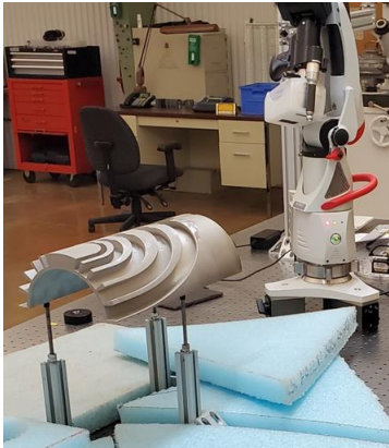
Laser Scanning measurements of surface deviation from CAD.
