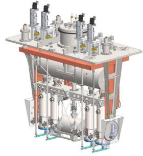
HL-LHC Crab Cavity Cryomodules
