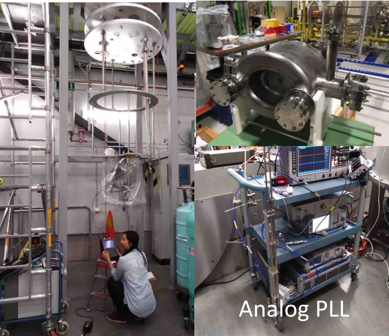
Double Quarter-wave (DQW) crab cavity
