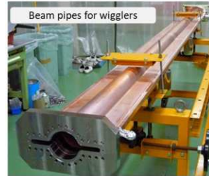
Beam pipes for wigglers
