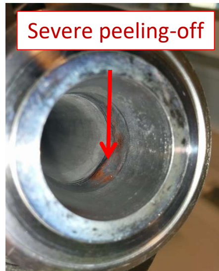
Peeling-off at RF fingers and Cu endpiece
