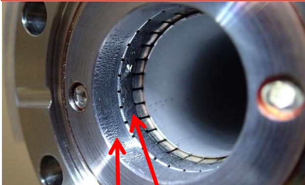
Peeling-off at RF fingers and Cu endpiece
