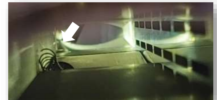
Ver Scraper: coil spring popped up
