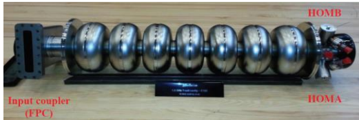
C100 cavity, and C100 cryomodule with FPCs in CEBAF section SL25, Jlab.
