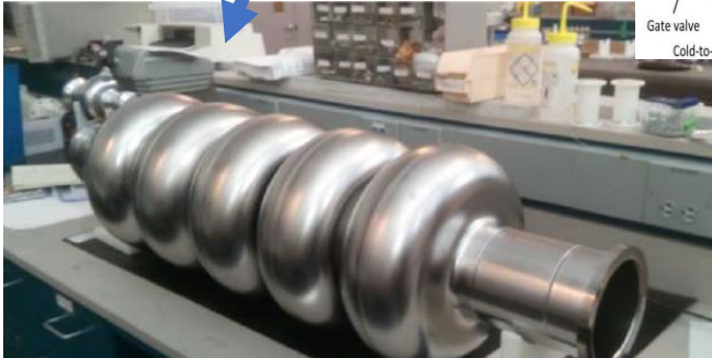
The first Nb 801.58MHz 5-cell elliptical cavity fabricated at JLab.
