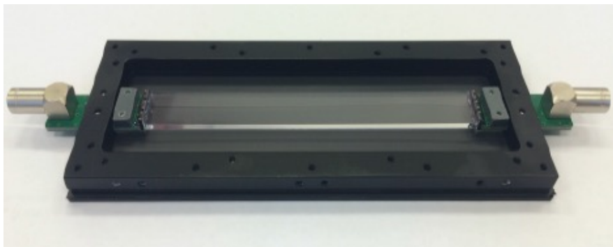
SiPM + 2 mm thin scintillators
