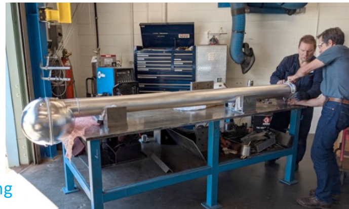
Challenging UCN source tail section wall welding completed, no leak test successful
