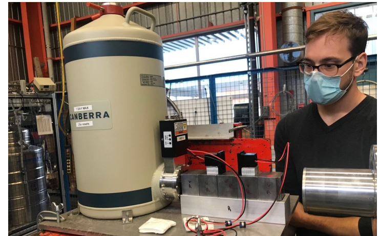
Preparing for installation and first tests of e-beam on tantalum foils in a prototype target chamber
