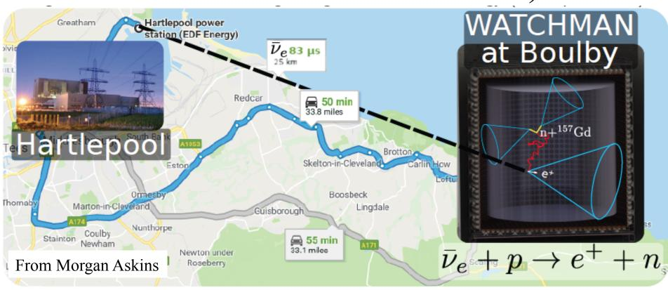
• WATCHMAN will demonstrate the ability to detect electron antineutrinos from a reactor from a significant standoff by the deployment of a 1 kiloton fiducial mass Gd-doped water Cherenkov detector in the Boulby mine – 25 km from the Hartlepool reactor complex in NE England.
