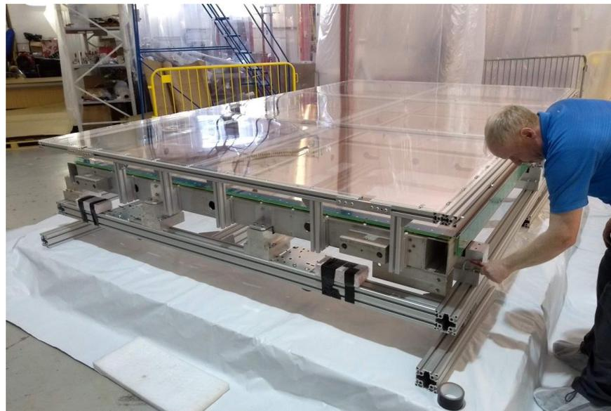
APA (anode plane assembly) prior to shipment to Fermilab from UK
