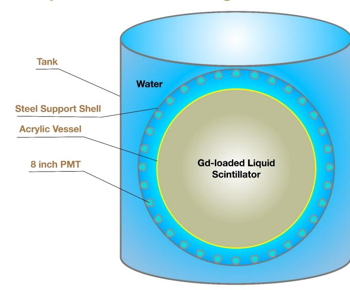
With the primary physics goals for geo-neutrino detection, the 200ton detector design follows the structure adopted by the recent underground neutrino experiments, and it will also consider the unique features of the low environmental backgrounds and the tunnel structure.
