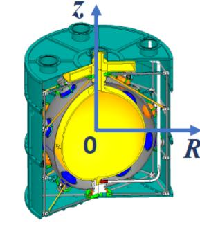
The deviation of Bi214 vertex distribution in Z-axis from origin indicates that air leak from top filling and instrument pipes.
