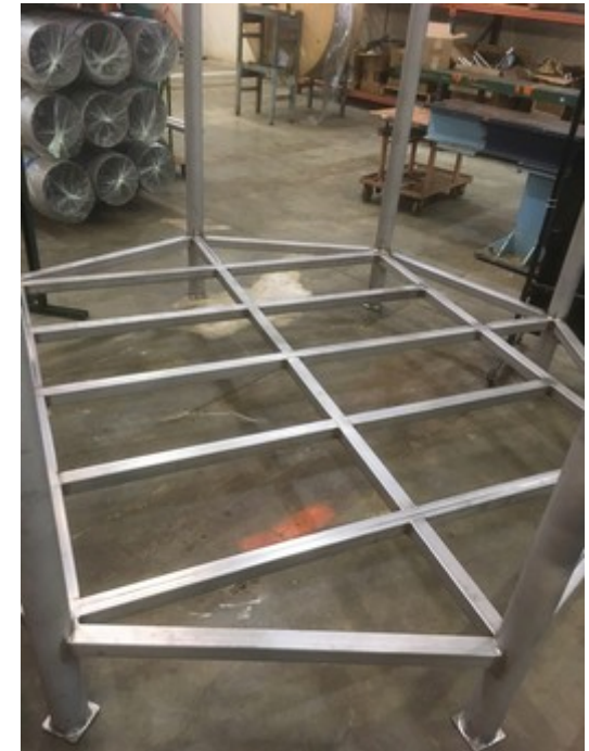
Stainless steel inner structure being welded and mounted!
