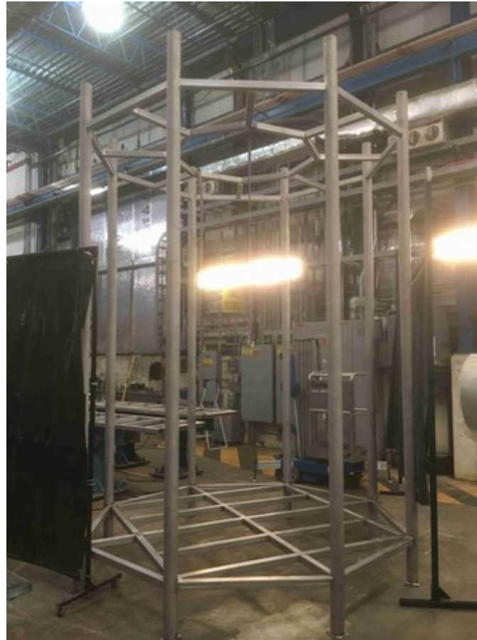
Stainless steel inner structure being welded and mounted!
