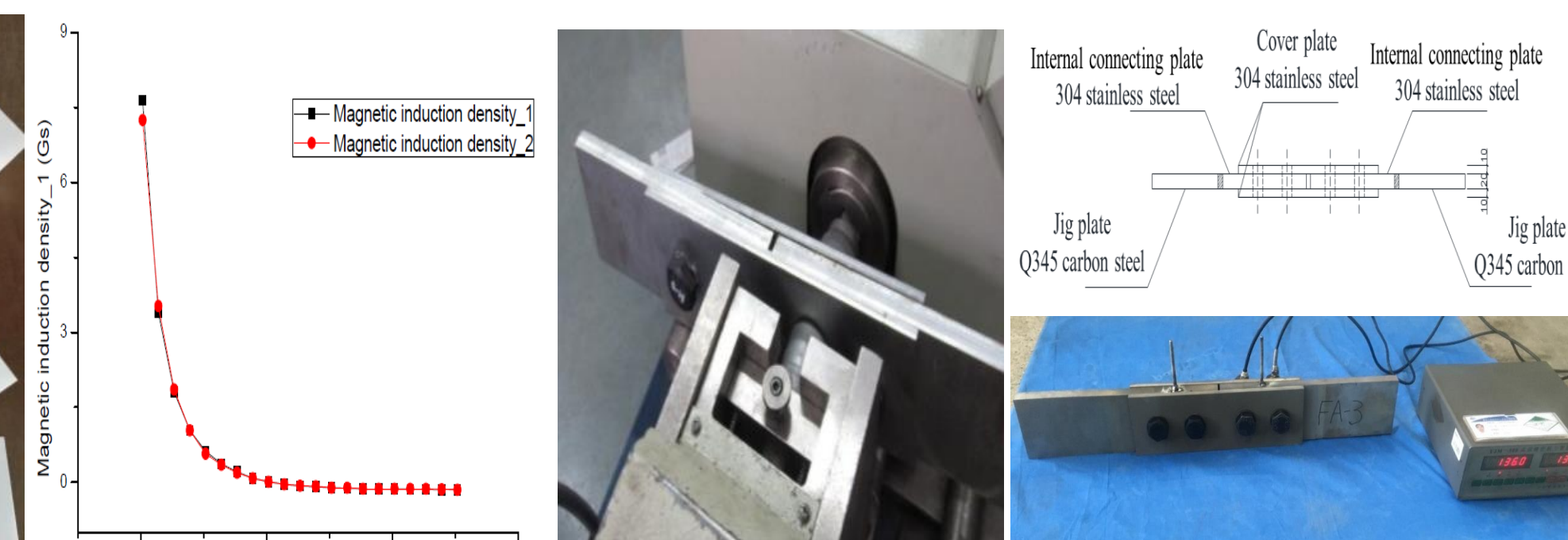
High-strength bolts and slip coefficient test
