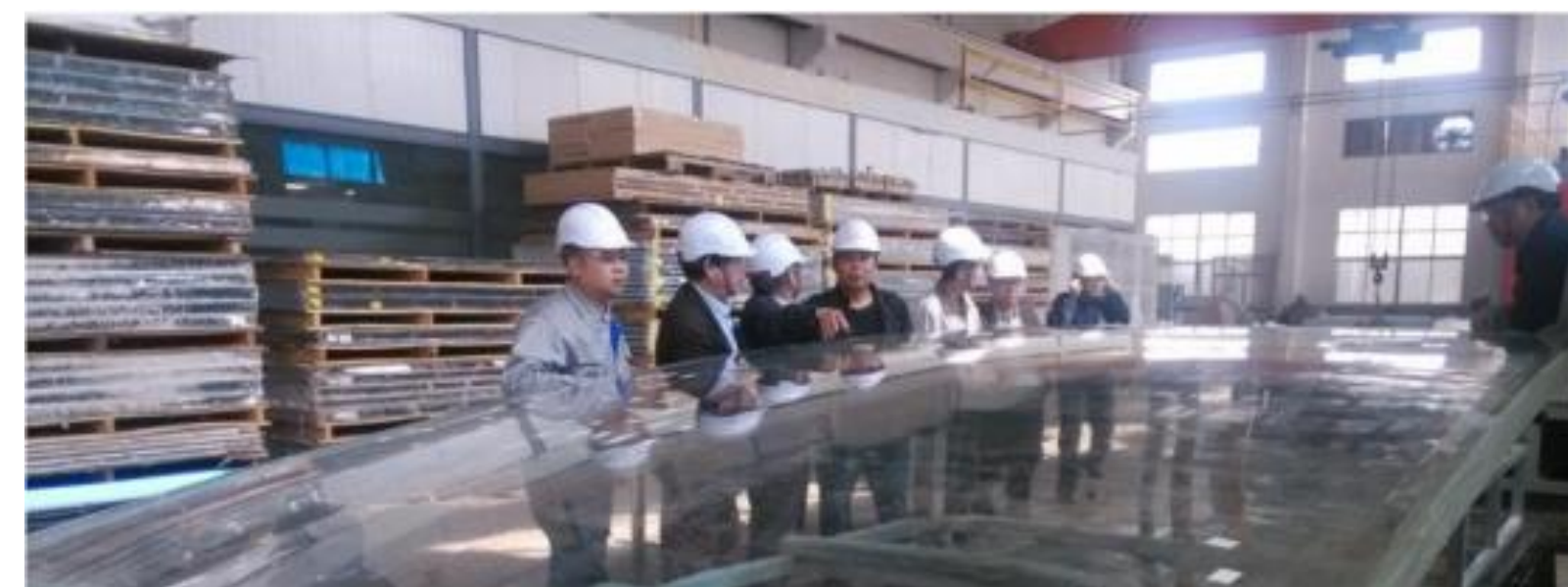
Thermoforming the spherical panel: 3m x 8m x 120mm
