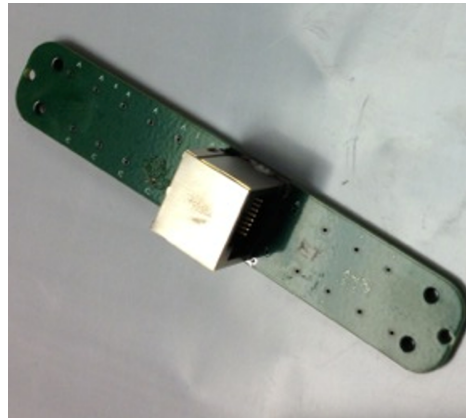
SiPM board with array of 12 SiPMs and RJ-45
