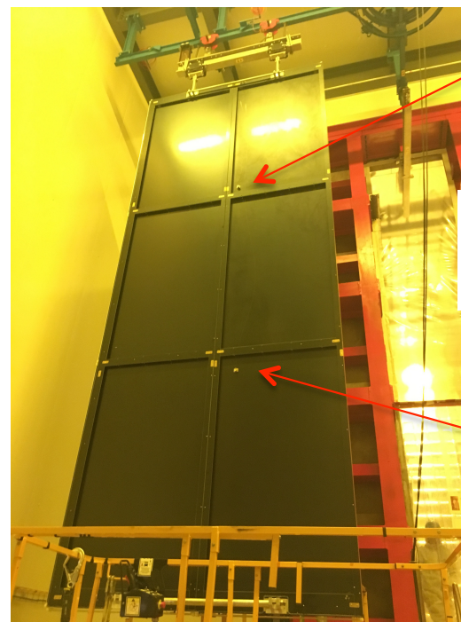
Pictures of light diffusers and fibers integrated with one CPAs at CERN.
