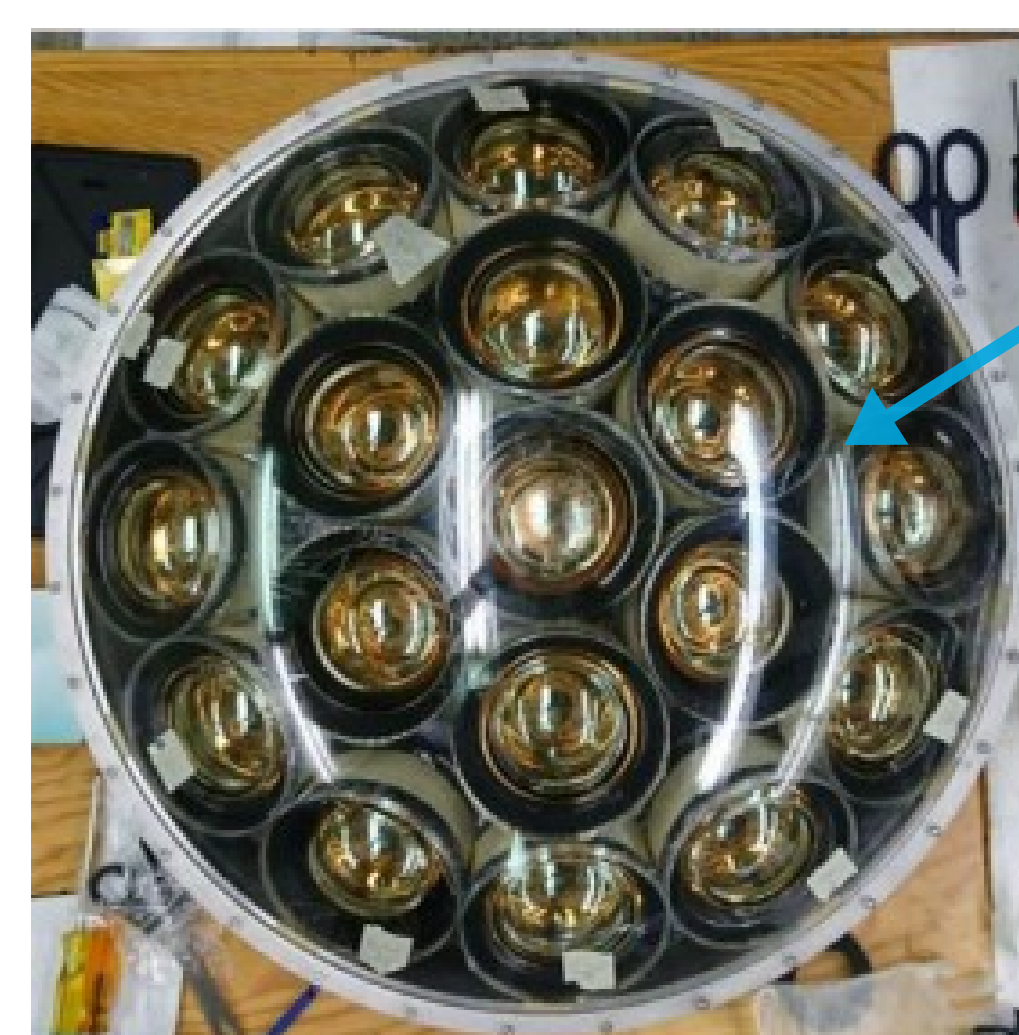
New photo sensor module - 19 3-inch PMTs/module
