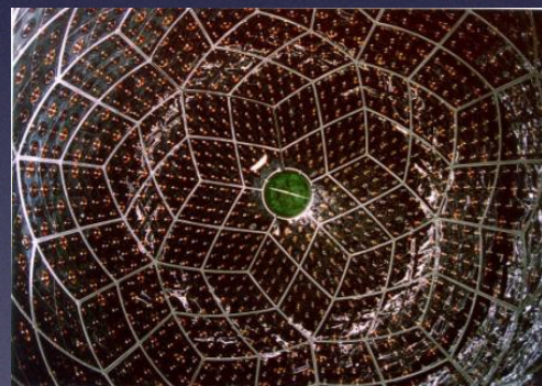
Liquid Scintillator 1 kton, 1900 PMTs (2002)
