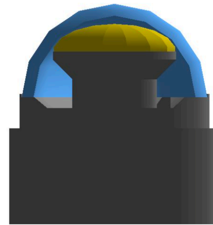
SDOM PMT housing Geant4 model
