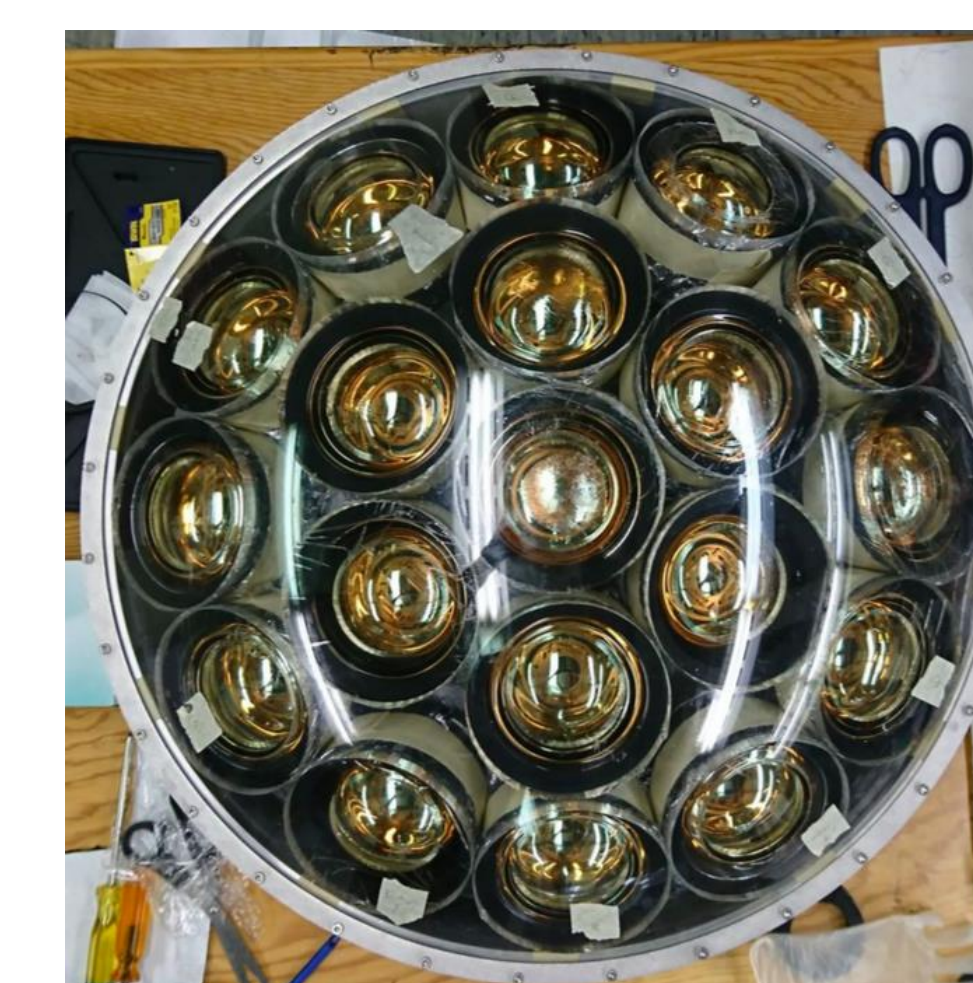
The multi-PMT prototype designed and built at TRIUMF
