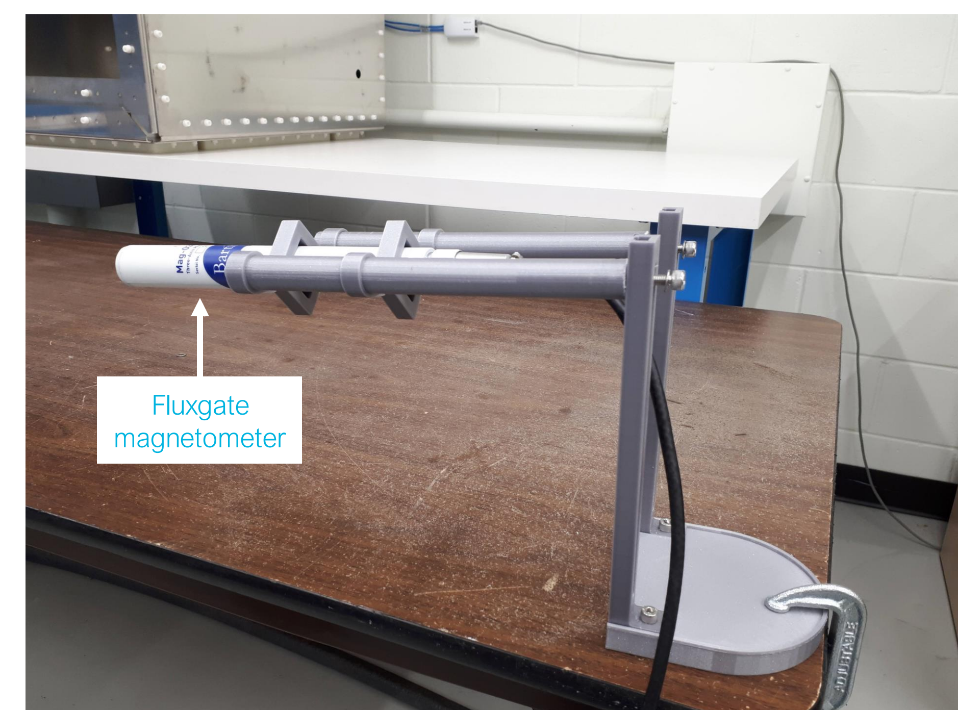
Figure 5: 3D printed custom fluxgate stand to be used in the Gradiometer shielding factor measurement.
