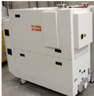
4 Busch combi DS3010-He pumping units specified and installed (1.4g/s @ 24mBar each)
