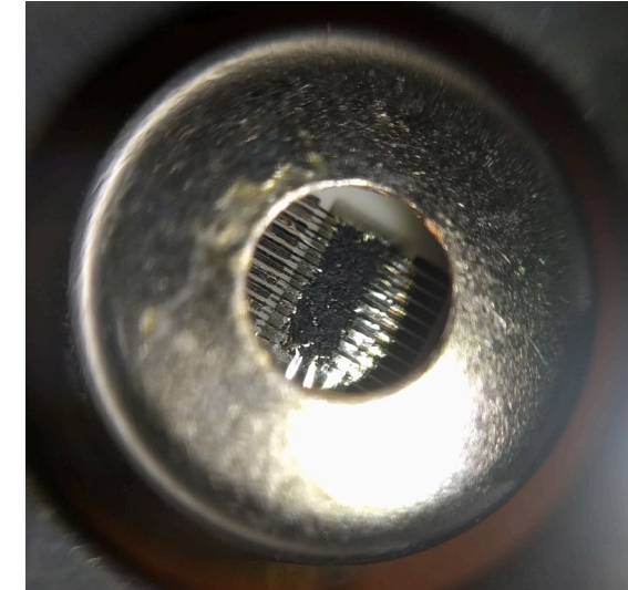
Thermopile detector used as temperature monitor
