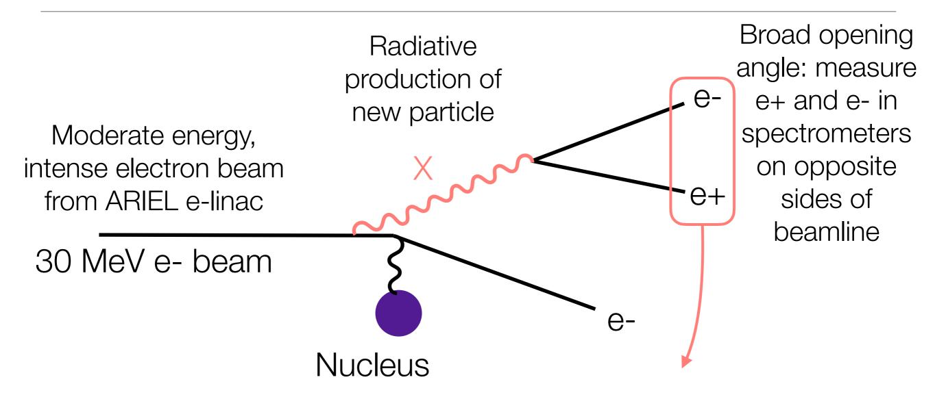
Dense target optimised for minimum multiple scattering
