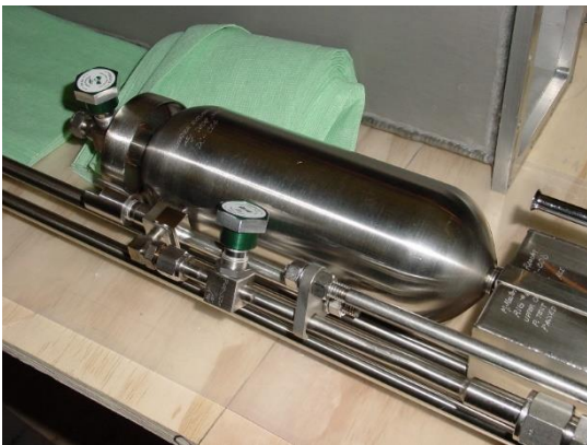
Xe-124 loaded into cylinder
