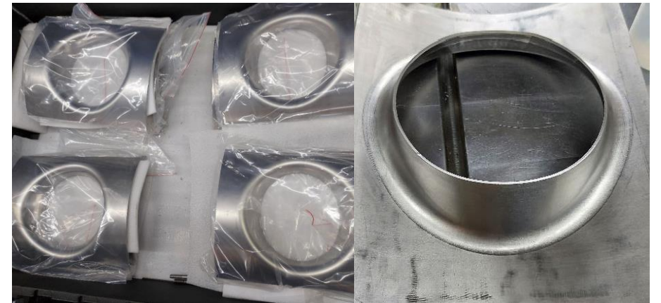
Production of pre-series single spoke cavity parts is ongoing at RI (DE)
