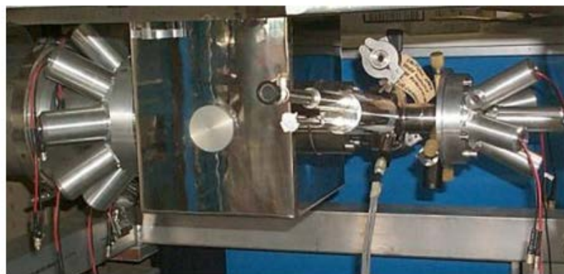
Muon & Active Collimator Detector Array Compact 7T Magnet 1.6K Cryostat Positron & Muon-Veto Detectors
