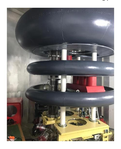
Low energy, high current accelerator for n-production for BNCT
