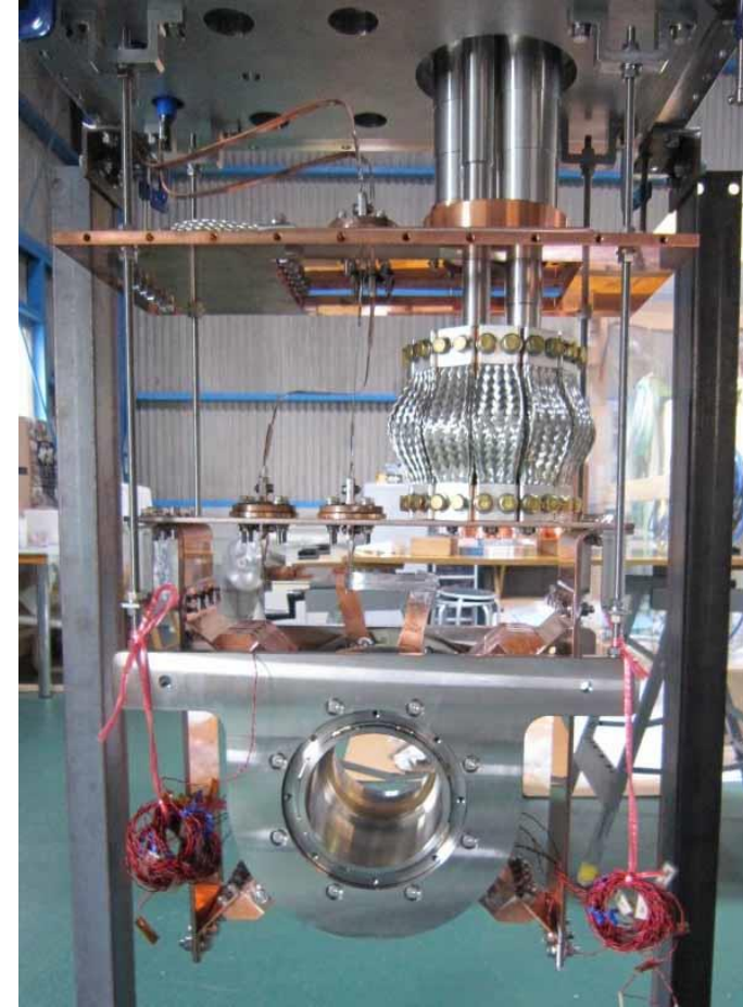
Connection to the 1 st and 2 nd stage of the pulse tube cryocooler.
