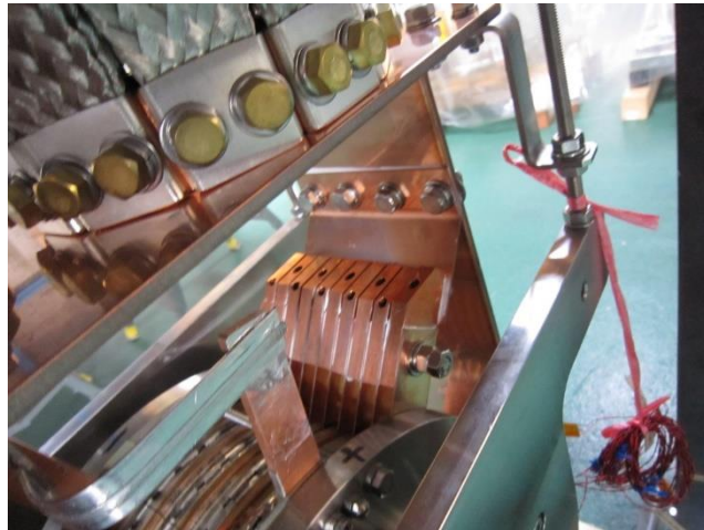
Coil and connection to current leads and cooling plates.
