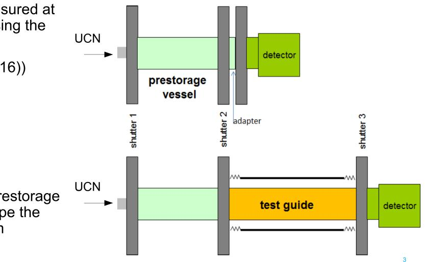
The method uses a prestorage vessel in order to shape the UCN energy spectrum
