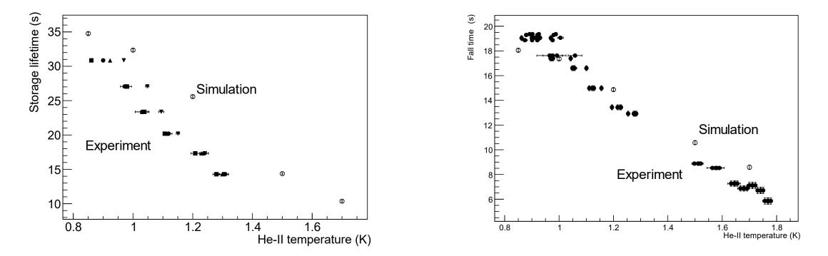
No helium vapor in simulation! Has significant influence at higher temperatures
