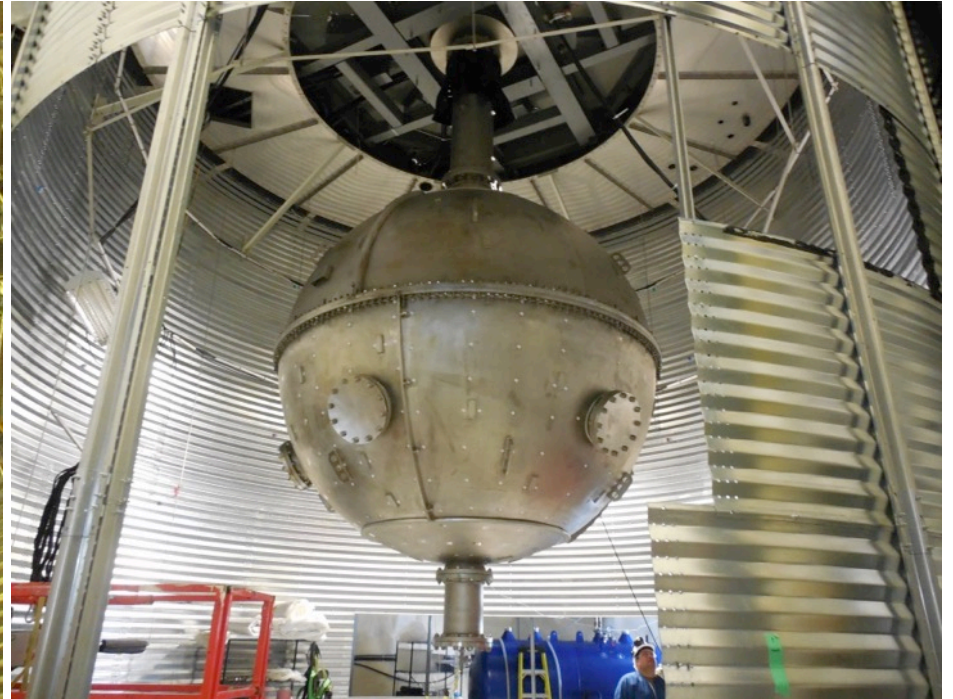
Steel Containment Sphere in 8m diameter water shield tank
