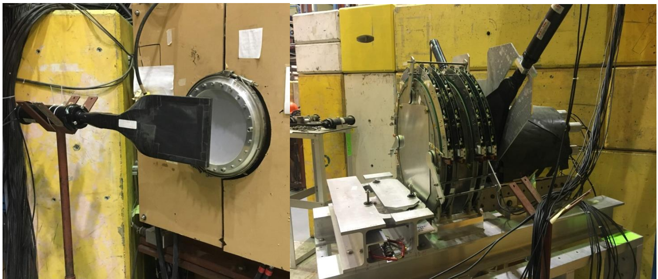
Figure 1: Left: View of the BC1 scintillator outside the beam port. Right: View of the drift chambers, BC2 and BC3 scintillators, and NaI crystal on a table in the M11 area.
