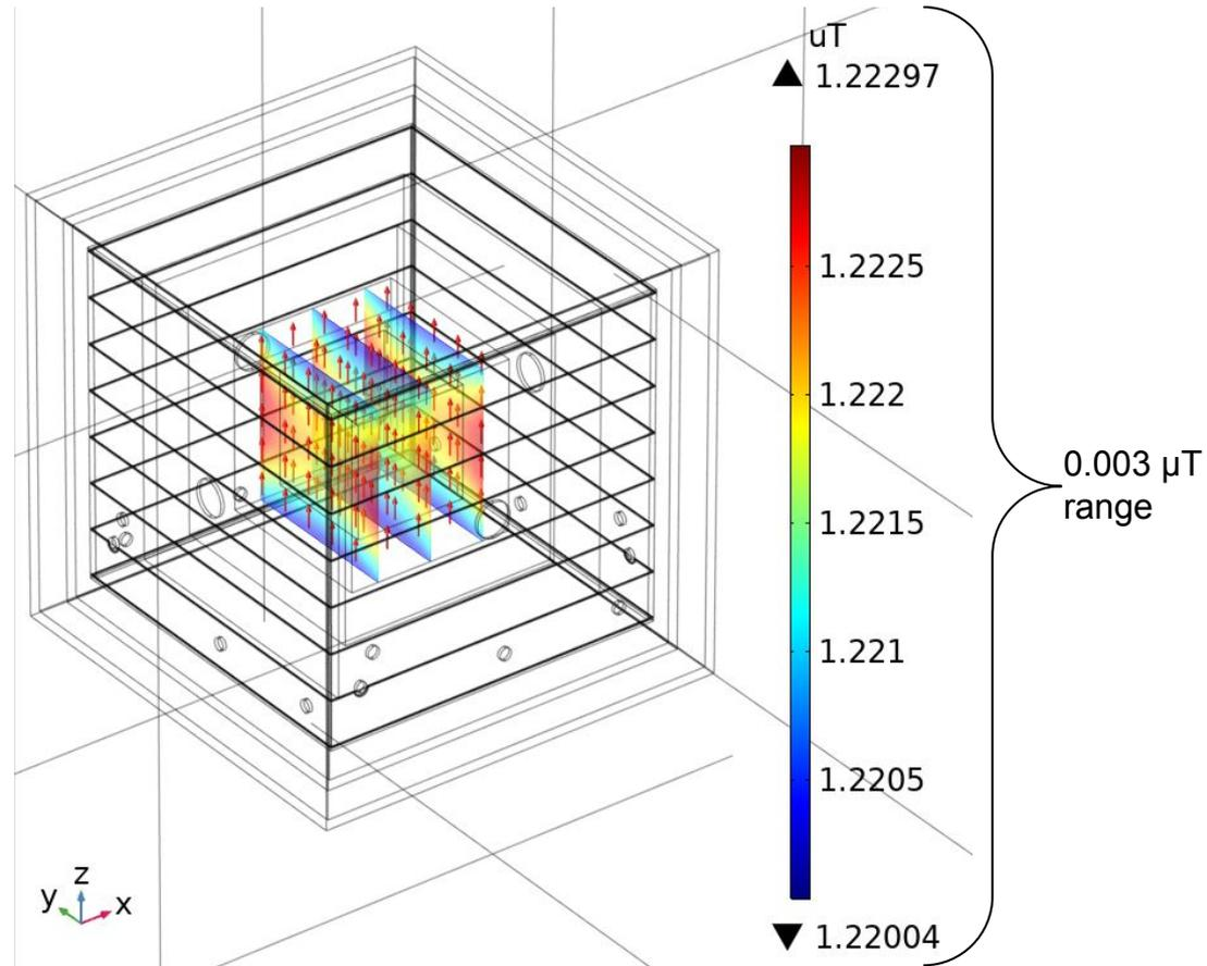
COMSOL simulation of 8 loop coil inside two layers of mu-metal, shown is the  $B_z$  field component
