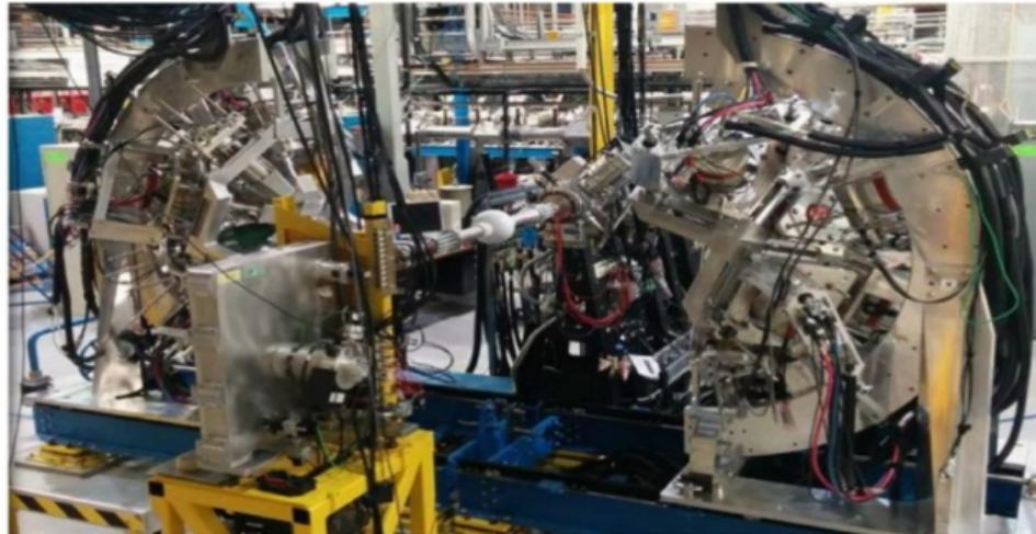
Both hemispheres of the GRIFFIN array showing the beamline and central vacuum chamber encased in a white 20 mm plastic delrin absorber.
