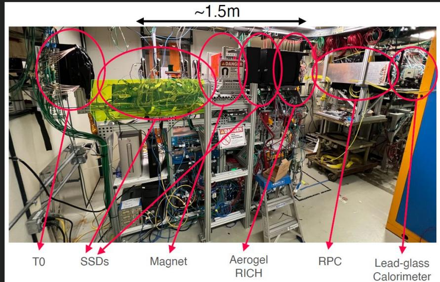
The **EMPHATIC** collaboration has been operating a compact experiment at **FERMILAB** Measurement of hadron production cross sections that are particularly relevant to neutrino flux predictions and not possible in other experiments.
