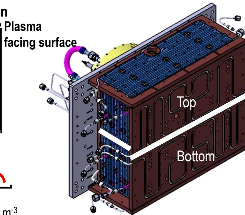
Vessel designed to have walls vertically split and all electrically independent and bias applicable:
