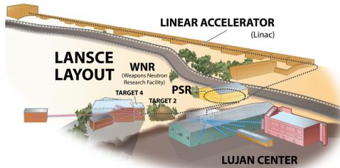
The Los Alamos Neutron Science Center (LANSCE) linac provides 800-MeV pulsed proton beams to produce spallation neutrons.
