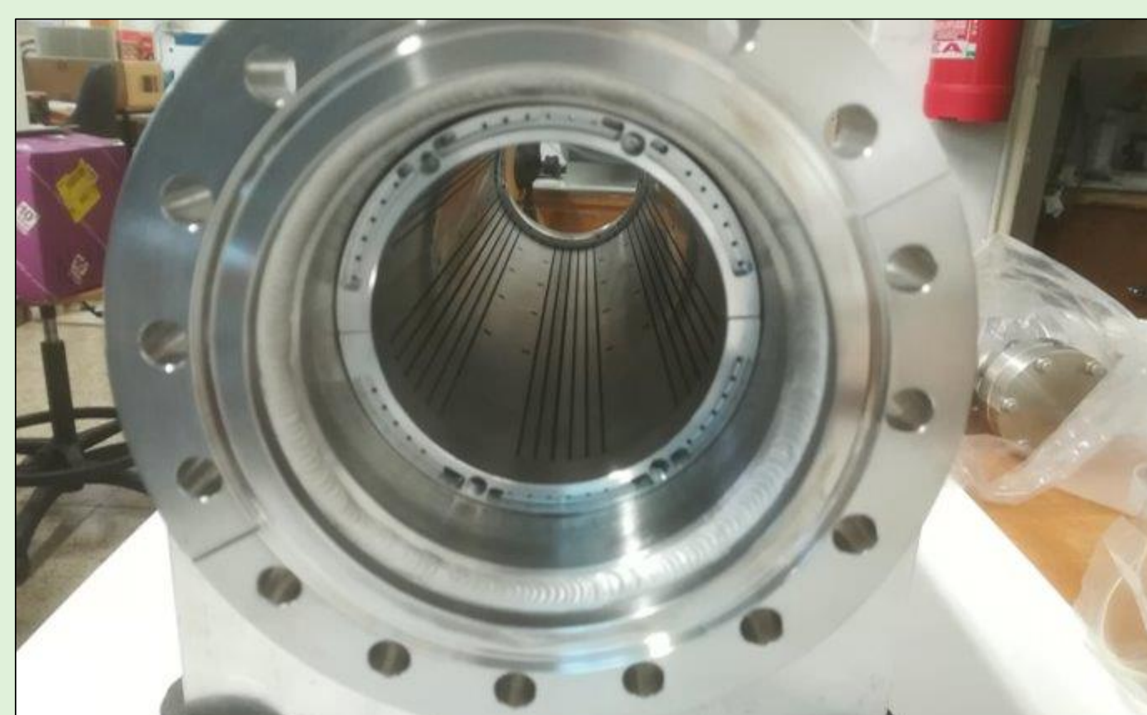
Wiring channels machined on the two half-shells.
