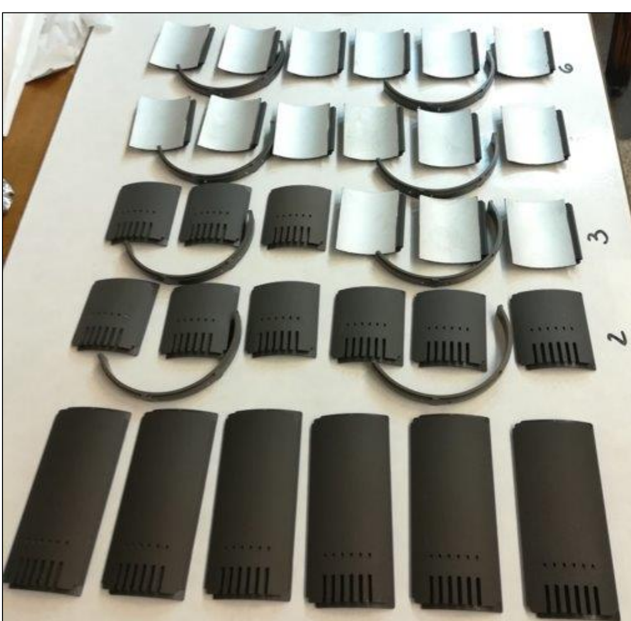
View of the 30 anodized tiles ready for installation in the active plasma chamber.
